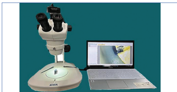
[Table/Fig-6]: Stereomicroscope*. (*Stereo Zoom Microscope Make: ACUCAL- PEEK coping being evaluated under a stereomicroscope at 60x magnification).
